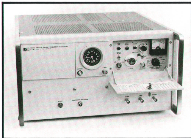
Fig. 1. HP 5061A Cesium Beam Frequency Standard is now available with standard or new high-performance cesium beam tubes. The high-performance tube's specifications guarantee 30% better accuracy, ten times better short-term stability, seven times better settability, and a factor of ten reduction in sensitivity to external dc magnetic fields.
